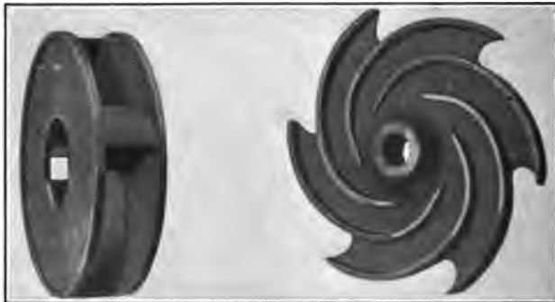
Sand pump impeller.
